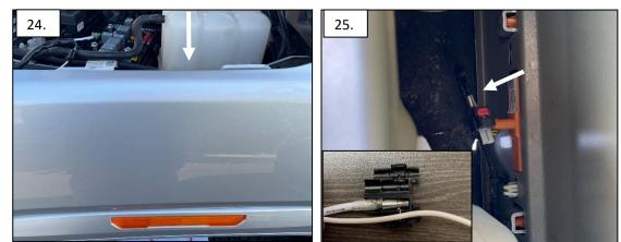
Tie all wires away from sharp, hot, and/or rotating components. Re-torque all the fasteners after 100 miles. Your install is now complete! Thank you for choosing Baja Designs.
